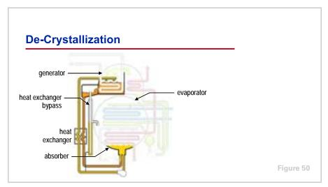
As a second line of defense, most absorption water chillers include devices that allow the chiller to recover in the event that crystallization does occur. Some of these devices simply sense impending crystallization, put the chiller through a dilution cycle, and shut the chiller down. Other devices keep the chiller operating while regaining control of the solution temperature and concentration.
